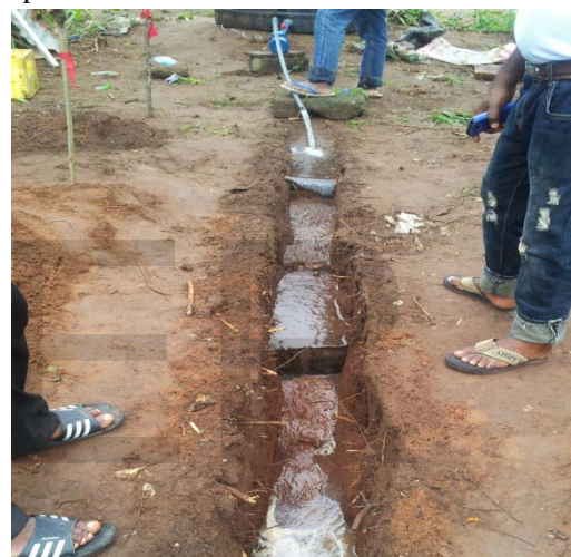
Plate 3: Experiment in progress, the water is being pumped from the tank, pressurized with the help of pressure pump of 0.5 horse power (hp)
