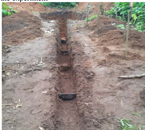
Plate 2: The excavation of artificial gully and inserted metal plates (check dam) ready for experiment.
